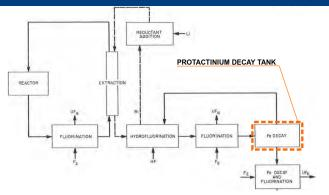
Figure: Protactinium isolation with uranium removal by fluorination [9].
