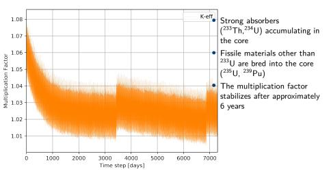
Figure:  $k_{eff}$  during a 20 years depletion simulation.
