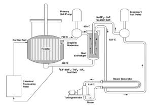
Figure: The MSBR [9] is an example reactor design with **liquid**, **mobile**, **circulating** fluoride salt fuel, including breeding behavior due to varying channel shapes and sizes. Image source [10].
