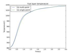
Figure: Fuel temperature rise following 1\$ ramp reactivity insertion, calculated with multipoint and single point kinetics in PyRK [15].
