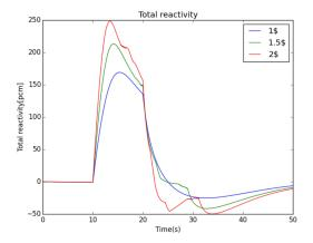
Figure: Total reactivity during ramped reactivity insertion as a function of inserted reactivity [15].
