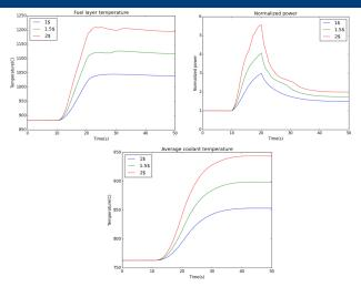
Figure: Average fuel temperature (left) and average normalized core power (right) during a ramp reactivity insertion in the PB-FHR [15].
