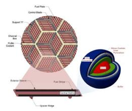
Figure: The AHTR [4] is an example of a fluoride salt cooled reactor design fueled by a **stationary**, **solid** prismatic graphite TRISO compacts, and cooled by clean fluoride salt. Image source [6].
