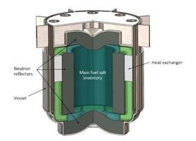
Figure: The MCFR from TerraPower is an example reactor design with liquid, mobile, non-circulating chloride salt fuel. Image source [14, 2].
