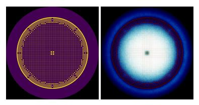
Figure: Above, full MSBR core neutronics simulation in Serpent (Rykhlevskii et al. 2019 [12]). Left: geometry. Right: Monte Carlo Neutron Transport scattering and fission.
