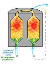
Figure: The pebble fuel can be assumed approximately stationary, as their movement is not comparable to the longest precursor decay times.
