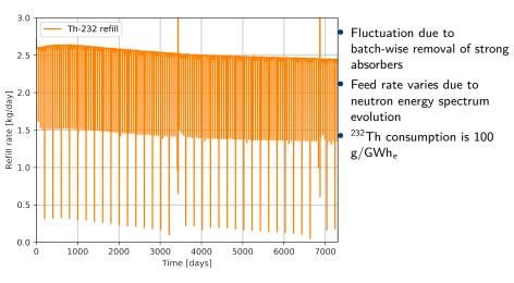
Figure: <sup>232</sup>Th feed rate over 20 years of MSBR operation
