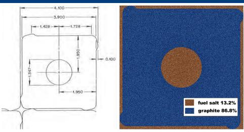
Figure: Molten Salt Breeder Reactor Zone I unit cell geometry from the reference [8] (left) and SERPENT 2 (right).
