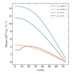
Fig. 12. The thermal and fast flux profiles at the core mid-plane (z = H/2) for the Moltres 2-D cylindrical axisymmetric model and the MSRE design model (Briggs, 1964, p. 92) (r = 0 is radial center of core).
