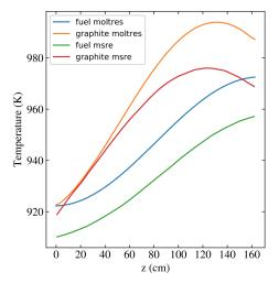
Fig. 11. Moltres and MSRE design (Briggs, 1964, p. 99) predicted axial temperature profiles in hottest channel and adjacent graphite.
