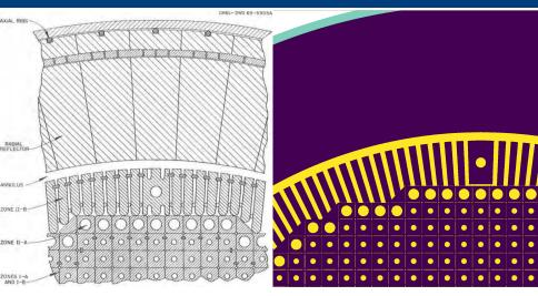
Figure: Detailed plan view of graphite reflector and moderator elements.
