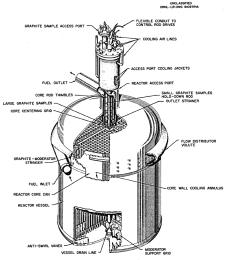
Fig. 6. MSRE Reactor Vessel.
