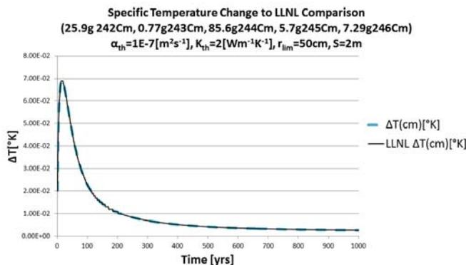
Fig. 3: This comparison of STC calculated thermal response from Cm inventory per MTHM in 51GWd burnup UOX PWR fuel compares favorably with results from the analytical model from LLNL.
