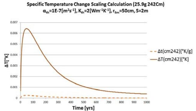
Fig. 1: As a demonstration of the calculation procedure, the temperature change curve for one initial gram of  $^{242}\text{Cm}$  and is scaled to represent 25.9g, approximately the  $^{242}\text{Cm}$  inventory per MTHM in 51GWd burnup UOX PWR fuel.
